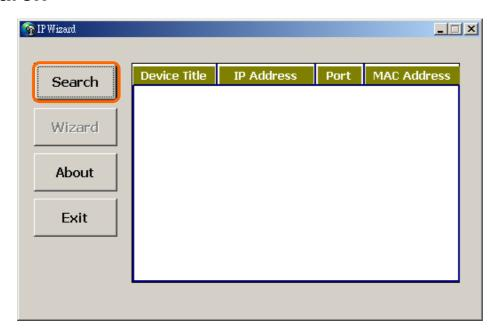
When click **Search** button, a searching window will pop up. IPWizard is starting to search Network Cameras on the LAN. The message "No Network Camera Is Found" will appear on this window if IPWizard can not find any device on the LAN. Otherwise, existed devices will be listed as below.
